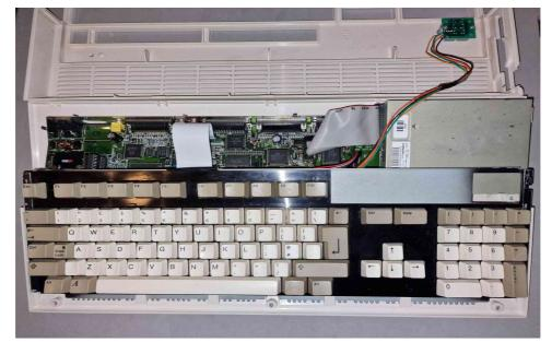
3. Lift the keyboard tab connector first before removing keyboard flexible tape. Now you can remove the keyboard.
