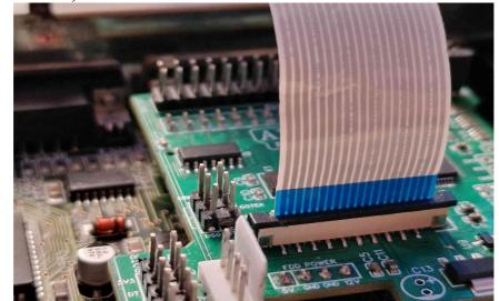
11. Reconnect 34 pin data cable to the floppy drive and then to the **GoDRIvE1200** board (NOTE PIN 1 ON THE GoDRIvE1200 IS ON THE RIGHT HAND SIDE CLOSE TO THE FDD). Make sure it sits firmly. Now reconnect 4 pin power cable to the FDD first, then to the emulator board.
