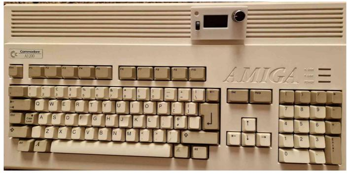
**Side note:** Due to the nature of 3D printing and the fact that you fit it on a 30 year old machine **discrepancies may occur**, therefore notches underneath breakout box are more likely for guidance only. I do recommend to use some sort of non invasive adhesive solution (double sided tape) to keep it in place.
