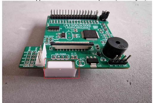
5. As GoDRIvE1200 sits directly on the FDD 34pin data socket: TAKE YOUR TIME, AND MAKE SURE IT'S ALIGNED CORRECTLY, AS ANY MISALIGNMENT MIGHT CAUSE DAMAGE TO THE EMULATOR/ MOTHERBOARD!!!
