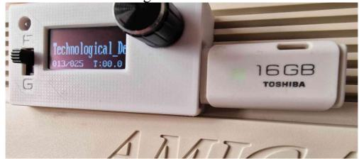
.ADF image names should appear on the screen. By using a rotary encoder choose which file you want to load and check if loading correctly.
