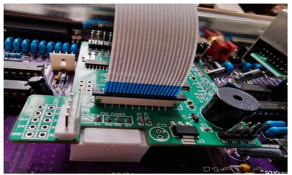
8.Reconnect 34 pin data cable to the floppy drive and then to the GoDRIvE1200 board (NOTE PIN 1 ON THE GoDRIvE1200 IS ON THE RIGHT HAND SIDE CLOSE TO THE FDD). Make sure it sits firmly.
