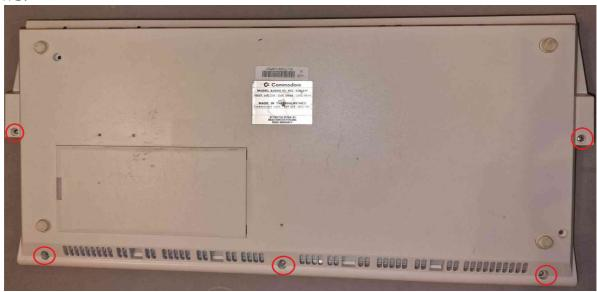
2. Turn it over and lift the top case and put behind as in the picture.
